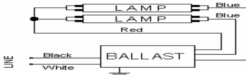
Note: For one lamp application, cap any blue lead. Insulate to 600 volts.
